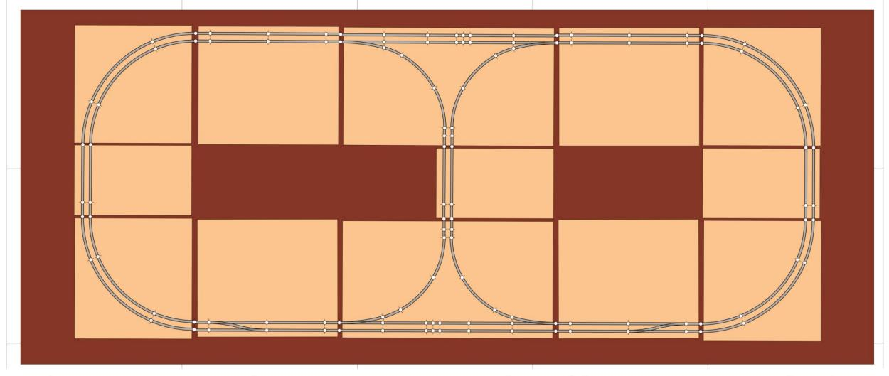
The brown area in these diagrams represents 4 six foot tables creating a 5 x 12 foot layout surface. With more tables more straight modules of any size could be added to the length. The use of 19 inch corners and/or branchline junctions allows for the creation of extra deep (20") straight modules of the standard T-TRAK lengths such as these singles and doubles.
