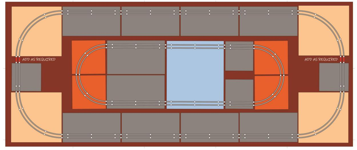
If you're going to use large radius corners with a bunch of standard size straight modules a second loop layout could be added inside the outer layout loop using standard corner modules. Any of KATO's small straight track pieces up to 64 MM or a combination of pieces as required by the size of the modules to accommodate the inside loop can be added.
