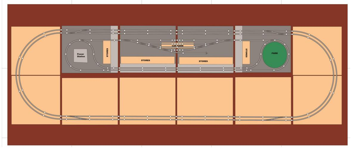
In my KATO Compact Track newsletter article I showed this trolley layout within a layout. The 20" depth of those modules was arrived at by accident trying to create the layout and were found to work well with 19" corners. Deep modules (over 14") are allowed in T-TRAK with skinny modules available for the other side of the loop, based on single table wide layouts. With 19" corners even deeper modules could be accommodated the same way.
