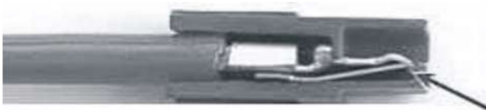
Figure 48: Releasing a contact in a Powerpole connector
