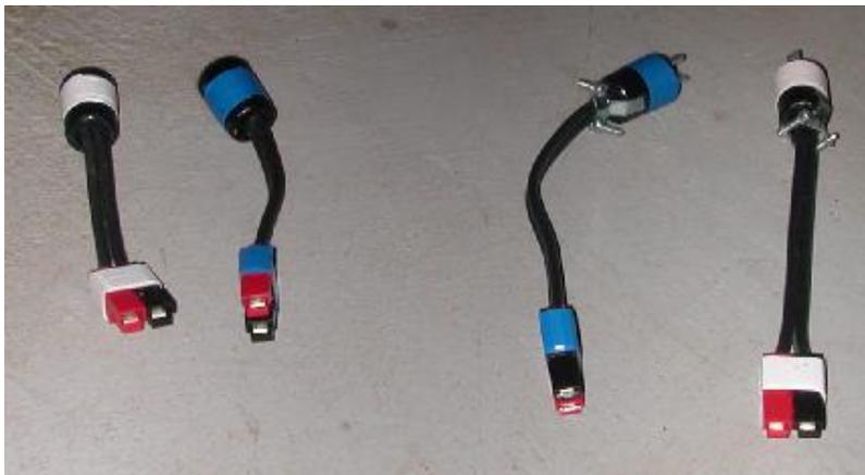
**Figure 7 – Track Bus and Power Bus Adapters**
