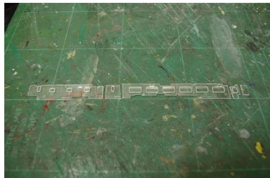
The glazing on the side to be altered needs to be cut up thus, then put away for safe keeping until reassembly time. The little window in the middle is now surplus.
