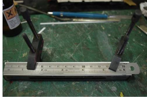
Short pieces of the skirt material are added at the ends to give some reinforcement (you can just see them in the next photo), then it's time to profile the skirts. This is done by rubbing them along a large flat file (the same one used to level the bottom of the original body in fact). The problem with this is that the sides are quite flexible, so a block of wood had to be cut to fill the body.
